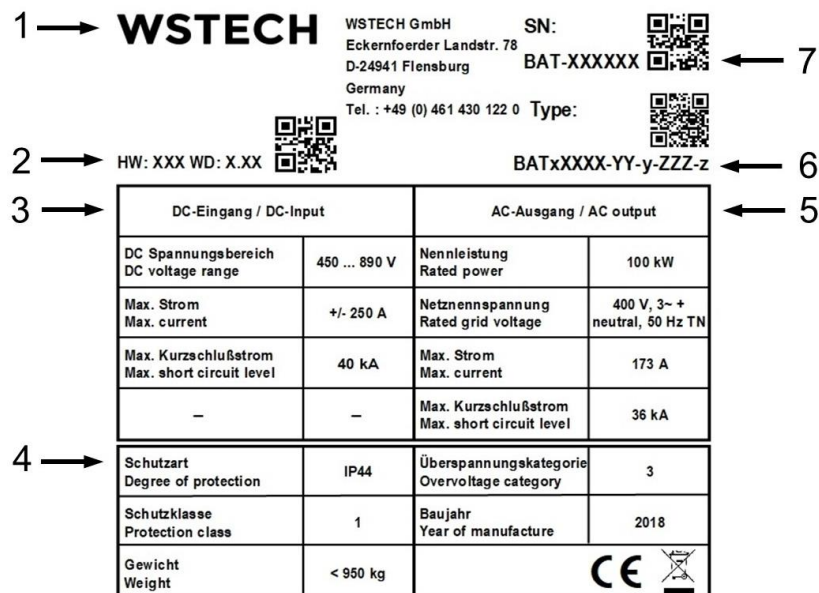
Figure 1: Example of a type plate
